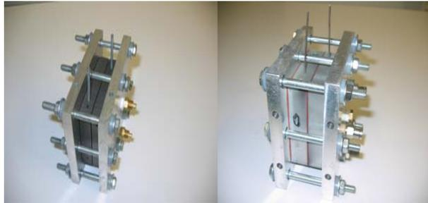
Graphite & Metallic Bipolar Plates Fuel Cells
