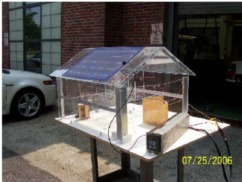
Picture 1: The dynoload on the picture was simulating a load that varies from 0 amps to 1.5 amps.
