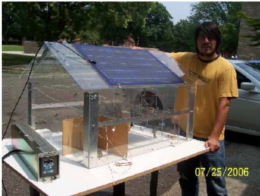
Picture 2: Here we see two solar panels of 15 watts output each that adds up to 30 watts total. These panels are located east-west for a better use of the available are of roof.
