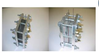
Graphite & Metallic Bipolar Plates Fuel Cells
